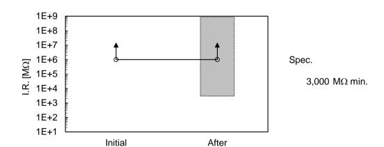
(Dielectric Strength) AC4000V(r.m.s.),60 s Dielectric Strength (Between lead wires) : No failure Dielectric Strength (Body Insulation) : No failure Appearance : No marked defect
